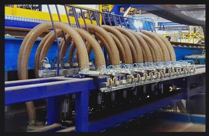
The NKE-PCS-5000 Plate Surface Cleaning System is intended for high-speed, in-line removal of dirt, dust, scale, and other foreign particles from the top plate surface.
