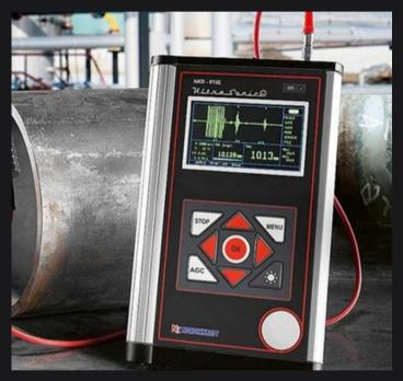
The NKD-019 Ultrasonic Portable EMAT Thickness Gauge is a convenient, compact, sophisticated, and innovative field instrument. This instrument can be used to measure the thickness of components, pipes, vessels, and other metal objects easily and precisely. The gauge enables measurements to be taken at a vast range of surface temperatures, going from -20 to 720 degrees Celsius. As a rule, plastic coatings, paint, or limescale on the surface do not affect the results of measurements.
