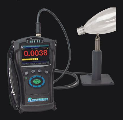
The MTG-99 Magnetic Thickness Gauge Series offers user-friendly NDT measurement for non-ferrous materials up to 1" thick with access to both sides. The flagship MTG-99 model is portable, battery-operated, features color change and vibration for alarms, and can include an optional internal datalogger.
