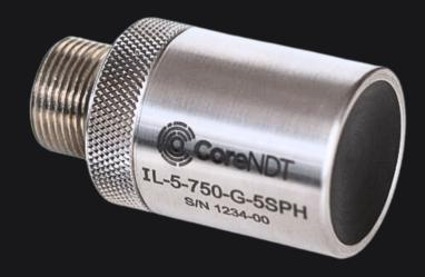
The Large Diameter Immersion Transducers are designed to be watertight and operate underwater. They have an impedance matching layer which helps to allow more sound energy into the water which continues into the part being inspected.
