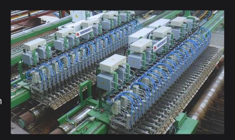
The Ematest-PL is an innovative, fully automated, in-line nondestructive testing system. It addresses material condition assessments of metallic plates, coils, welds, skelp, and many more by using UT, EMAT, and/or ET methods. 100% of production is inspected, providing valuable information for grading, quality inspection requirements, and process control data nearer to the process to reduce scrap rates caused by process errors.
