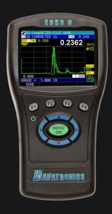
The **Echo 9 Series Corrosion Thickness Gauges** are advanced thickness gauges that comes equipped with a 3.5" high-resolution sunlight-readable color display, offering live A-Scan, echo-to-echo capability for coating detection, B-Scan functionality, a datalogger with up to 32GB SD card storage, and compatibility with Microsoft Excel.
