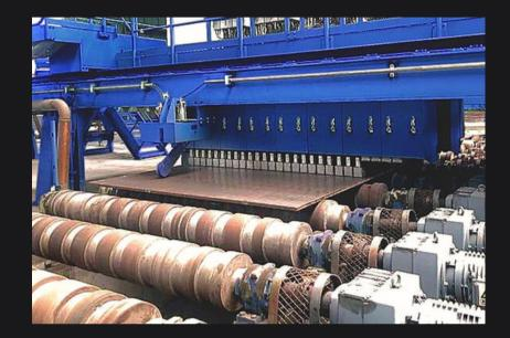
The EddySpot-PL detects hard spots are areas with irregular hardness normally occurring on the production line from the hot rolling process of plates, also referred to as bruises. These areas of local hardening variances become a source of mechanical stress after forming plates into line pipes (LSAW or HSAW).
