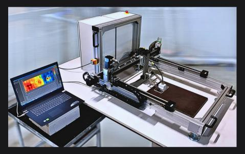
The EddySpot-Desktop detects hard spots, areas with irregular hardness normally occurring on the production line from the hot rolling process of plates, also referred to as bruises. These areas of local hardening variances become a source of mechanical stress after forming plates into line pipes (LSAW or HSAW).
