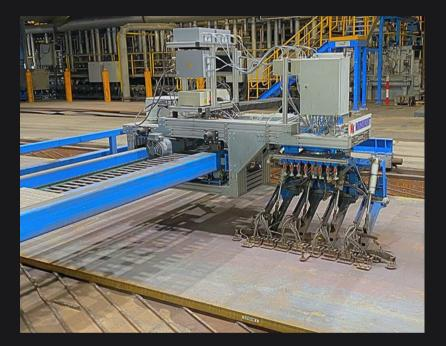
The EddyScan-PL detects hard spots are areas with irregular hardness normally occurring on the production line from the hot rolling process of plates, also referred to as bruises. These areas of local hardening variances become a source of mechanical stress after forming plates into line pipes (LSAW or HSAW).
