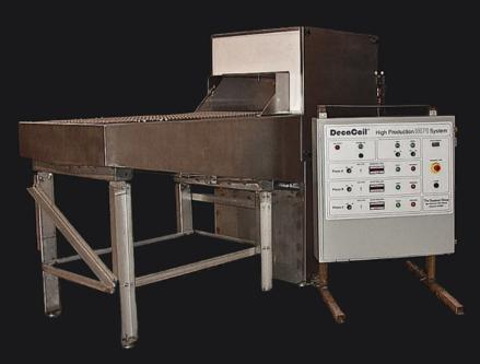
The DecaCoil High Production MPI System is a non-contact, multidirectional, induced MPI system with automatic bath application and a motorized conveyor. The basic scheme of operation requires the loading of test components onto the motorized conveyor either manually or by means of plant robotics or conveying systems. These components are transported into the magnetizing tunnel, where they are sprayed with magnetic inking material and magnetized in three vectors simultaneously.
