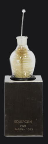
The Centrifuge Tube Set is used for the determination of content of solid particles in inspection carrier solution for magnetic particle examination. The concentration of particles in the suspension is a very important parameter in the inspection process and must be closely controlled.
