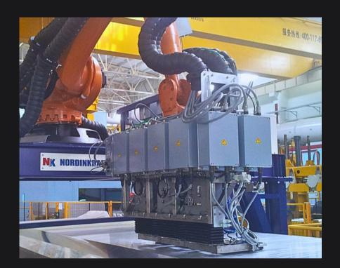
The Alutest-PL systems are intended for fully automatic ultrasonic and eddy current examination of plates and slabs made of non-ferrous metals such as aluminum, titanium, copper, etc.
