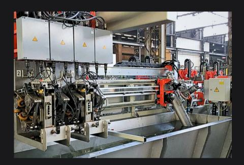
The Alutest-BB systems are designed for automatic ultrasonic testing of bars and billets made of aluminum, titanium, copper, and other non-ferrous metals. Like the Nordiscan-BB series, this system can be delivered in two different configurations.
