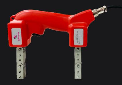
The Equipcon 7A Yoke is a powerful AC magnetic yoke used for detection of cracks on surfaces during magnetic particle inspection. It is portable, lightweight and has detachable power cords for efficient use. The yoke is chemical, oil and abrasion resistant and has articulated legs which can spread approximately 2.35-10.6 inches (60-270mm).
