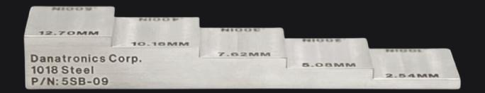
The **5 Step Test Block (#5SB-09)** is made of carbon steel which has English & Metric values engraved from 0.1" – 0.5" (2.54mm – 12.7mm).
