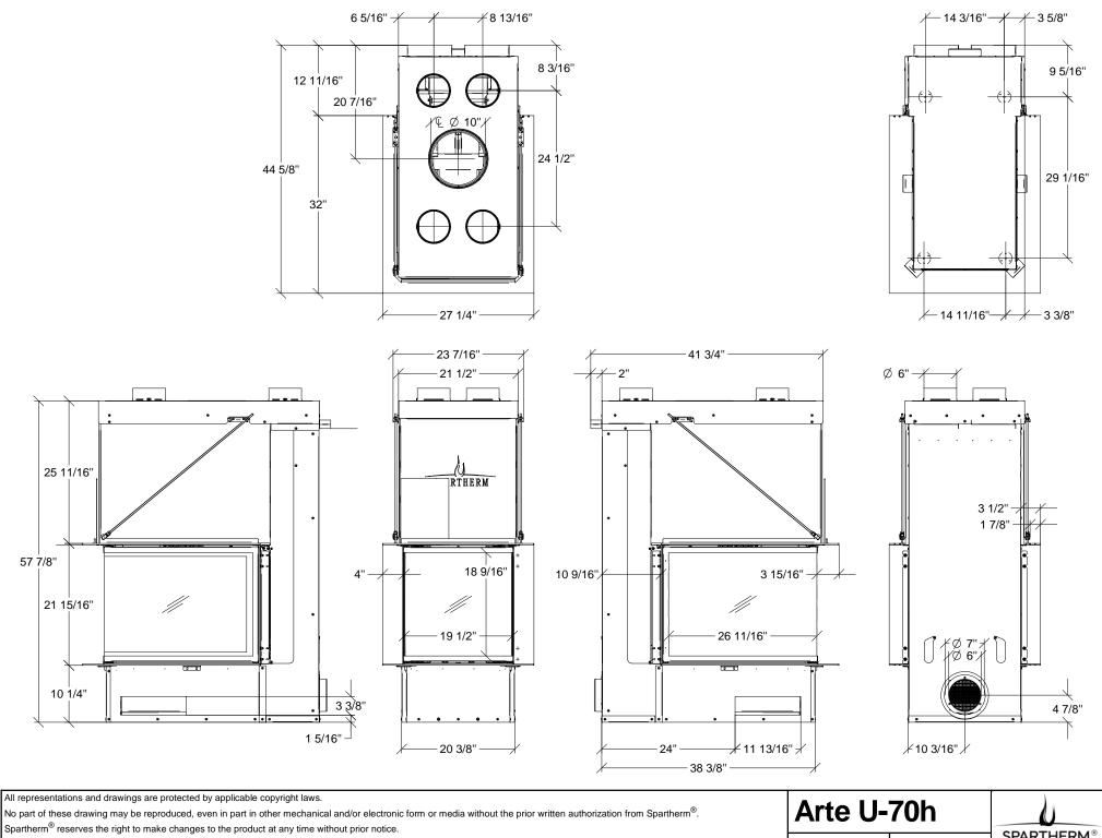
Unless otherwise noted measurements are in inches with a tolerance of ± 1/16". Spartherm® ©2022
