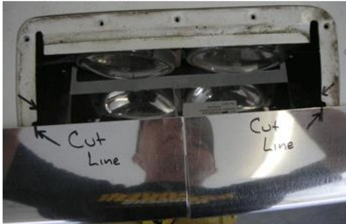
14. For Cessna 150 models trim the inboard 520 skin to length. For all other aircraft models NO trimming is required for the 520 skin. Correct length is dictated by having the proper overlap on the 524 inboard fairing, 5/8in. minimum, and aligning the outboard edge with the seam at wing station 84 for Cessna 150 models.
