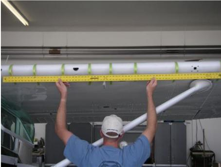
5. Mark the outline of the blocks and remove the blocks from the wing. Scuff the marked locations for the blocks on the leading edge to provide a rough surface for the adhesion of the silastic RTV. Clean surface again per process specification 732 if required.
