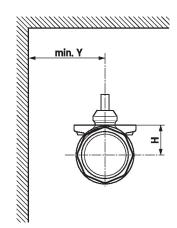
X/Y: Minimum distance with respect to the valve centre.
