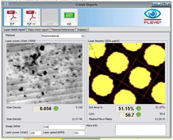
Click inside the Laser Power Image to start a Stain density measurement. The Reports window will close and the main BETAFLEX PRO application will automatically be set to Stain Density measurement. Zero and measure Stain as usual. The Result is automatically copied to the Reports Window. The Reports Window will automatically re-open.
