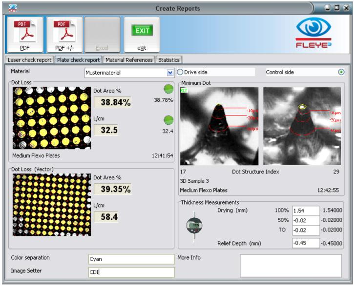
Click inside the Dot Loss Image to start a Dot Loss measurement on the Pixel variant of the 50% patch. The Reports window will close and the main BETAFLEX PRO application will automatically be set to dot area measurement. Measure the 50% pixel oriented patch as usual. The Result is automatically copied to the Reports Window. The Reports Window will automatically re-open.
