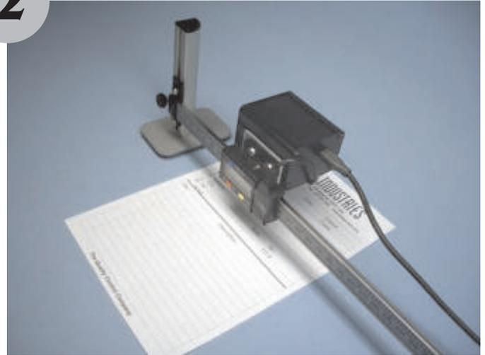
Place a sample of the material to be measured at the left end of the scale. Loosen the attachment screw slightly and slide the beam up or down to bring the image into sharp focus. Move the sample and camera to the right end of the scale and repeat the operation. The image will now be in sharp focus across the entire width of the device.
