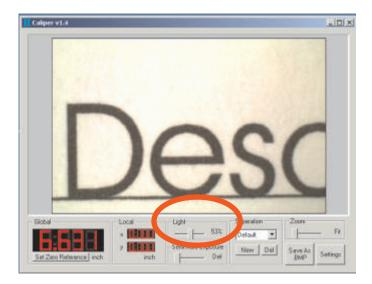
Both small and large objects can easily be measured using either the **Global** or **Local** mode of operation.
