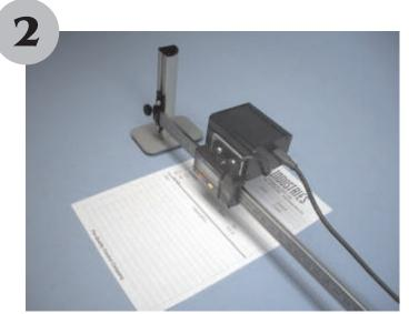
Place a sample of the material to be measured at the left end of the scale. Loosen the attachment screw slightly and slide the beam up or down to bring the image into sharp focus. Move the sample and camera to the right end of the scale and repeat the operation. The image will now be in sharp focus across the entire width of the device.
