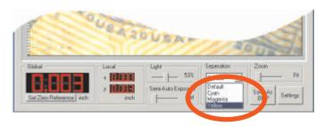
A high contrast monochrome image is now created, making the original pattern more readily visible. The low-contrast yellow pattern is now readily visible while the other colors are suppressed. The other process color filters are available and arbitrary spot color filters can be created.
