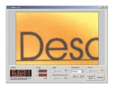
Raise or lower the horizontal beam on the vertical posts until the image is sharp at both ends of the beam. Move the **Light** control to about 50% as shown below.
