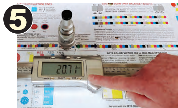
5 Turn the lower black ring to align the reticle
