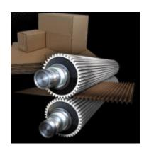
Today's practice of using carbon paper to check the condition of the corrugated rollers is not precise and can not be used to estimate how much corrugated can still be produced before the rollers have to be replaced.
