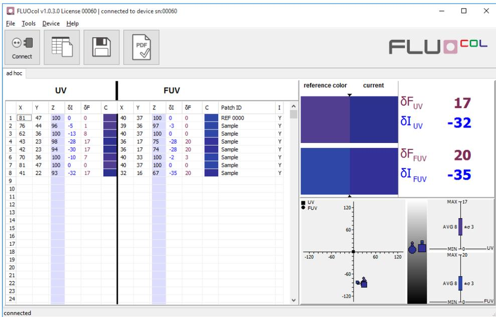
**Fig. 4 Beta FLUOcol software** display of Intensity differences of one ink in a production run. Data for near UV and Far UV measurements are collected in tabular form for export and further analysis. Where color is an important authentication factor, the Beta FLUO and FLUOcol software display the measured color and the Reference Color along with the calculated Intensity and Fluorescent Color differences.
