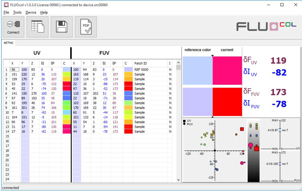
**Fig. 5 Beta FLUOcol software** display of Fluorescent Color Difference for multiple colors in a production run
