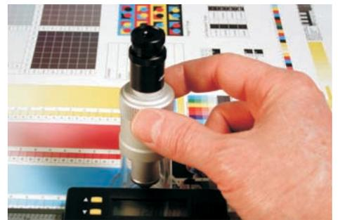
Bring the image into sharp focus by turning the large knurled ring.
