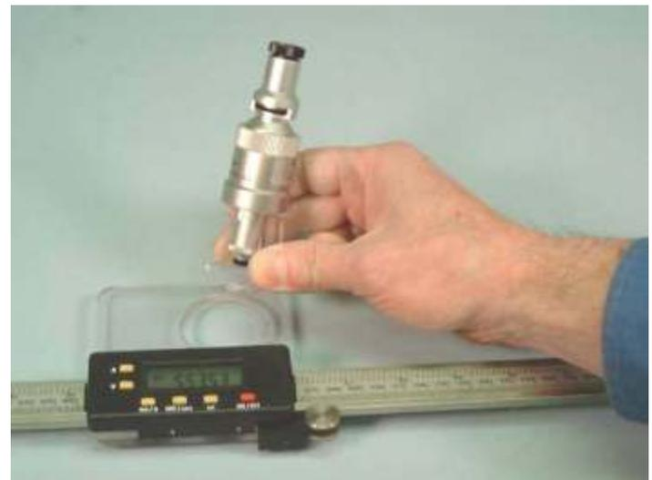
The microscope and digital readout should look like this after assembly. To remove the microscope when storing the ruler, squeeze the base and lift the microscope out.
