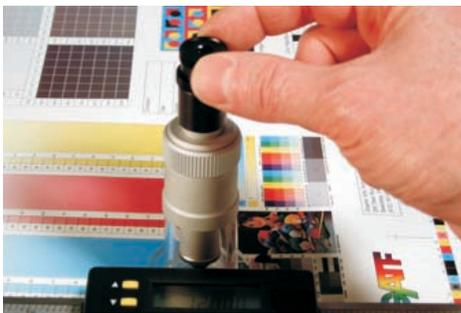
Rotate the upper black ring to bring the reticle into sharp focus.
