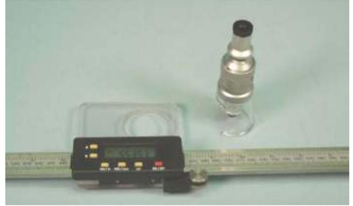
Squeeze the plastic base of the microscope as shown. Press one edge into the groove and then move the opposite edge into place. When properly seated, the microscope will be firmly held in place and will not fall out even if the assembly is inverted.
