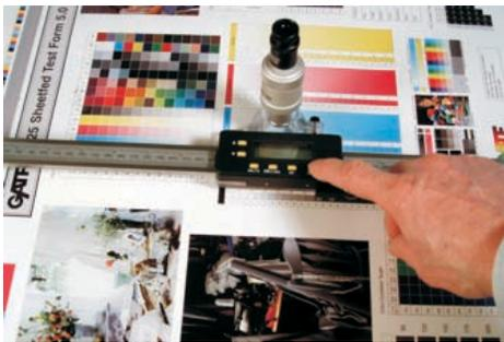
Press the red ON button to activate the display. Press the Inch/MM button to toggle between units.
