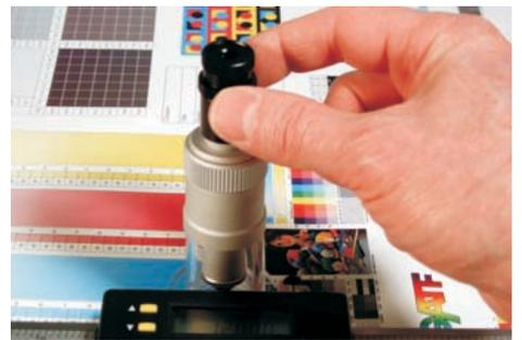
Turn the lower black ring to align the reticle to the image.
