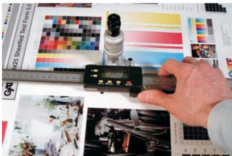
Slide the readout close to the end position and place in final position by using the fine motion roller as shown.
