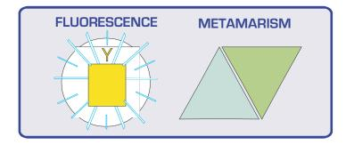
**FLUORESCENCE** in paper, inks, and coatings occurs when ultra violet light striking a surface causes it to emit longer wavelength light and resulting color shift.
