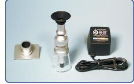
**OPTIONAL OPTICS** [10x, 20x, 25x, 50x, 100X] on interchangeable magnetic plates can be snapped on and off. This feature allows rapid interchangeability of optical magnifications without the need to refocus every time.
