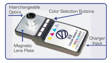
Pressing and holding any button will cause white LED's to illuminate the subject for general viewing. Releasing the button will initiate a specific color LED illumination.
