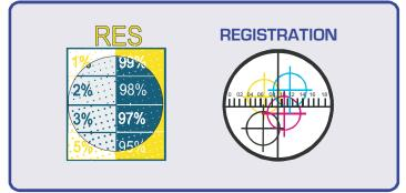
**RESOLUTION TARGETS** indicate the ability of the printing process to accurately reproduce the full range of dots from 1% to 99%. The BETACOLOR VIEWER can recognize errors at any source, whether it is film, plate or press.
