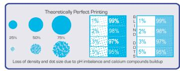
**CALCIUM CARBONATE** compounds deposits on plates, rollers, and blankets can cause poor ink transfer resulting in low ink density. First affected are disappearing highlight dots that are measurable with a press densitometer in the dot gain mode, but are better seen with the BETACOLOR VIEWER. Other factors are roller stripping, ink mottling, hickies, plate blinding, higher water speeds, ink emulsification, slow ink drying, and out of control conductivity and pH levels.
