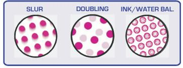
$\ensuremath{\textbf{SLUR}}$  can be caused by improper packing, worn grippers or a loose or stretching blanket.
