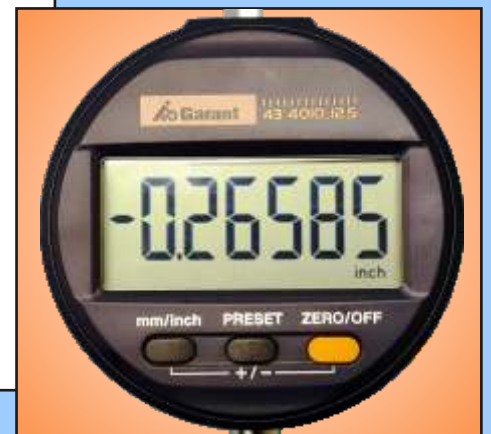
Digital Micrometer Reads to 1µ
