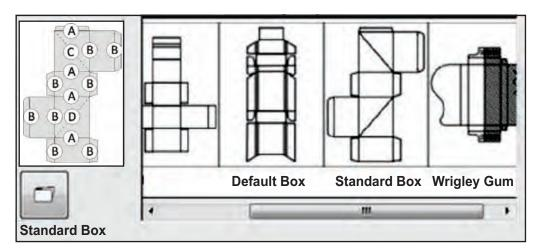
USING CUSTOMIZED BOX LAYOUTS To simplify when use a large number of boxes, the ADVANCED software stores box layouts graphically with their reference numbers. When a reference number is selected, the box's graphic image is loaded and displayed with it's measurement positions. The final report prints the customized box layout with the measurement data.
