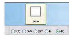
After the software installation, and before starting measurements it is necessary to zero the device on your substrate.
