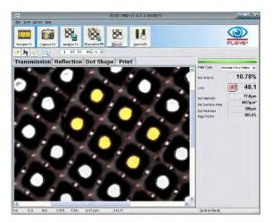
At least 3 dots adjacent to each other must be selected to obtain a correct result when using the Automatic or Fixed screen ruling function. Selecting more than three adjacent dots slightly improves the repeatability of the result by averaging more dot locations.
