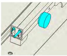
Make sure the Sensor connector is in the raised position by rotating the wheel clockwise on the right side of the support arm.
