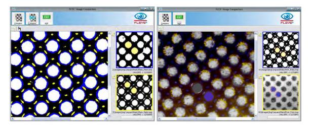
The blue areas surrounding the dots means that the blue image dots (ablation mask) are larger, showing the dot reduction between ablation mask and finished plate. Export the comparison image in JPG Format for documentation by clicking the save Icon.
