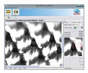
The dot diameter at different relief levels can be measured and a dot structure index is calculated and displayed.
