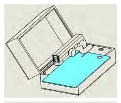
Open the device box and remove the large Plexiglas cover by sliding it to the front.
