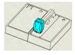
Connect the Sensor to the support arm by inserting the longer pin first and sliding it straight on until the shorter connector makes firm contact.
