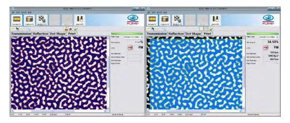
In order to maximize inter-instrument agreement between BETAFLEX devices and to improve the absolute accuracy, the BETAFLEX software always picks printing area elements within a constant area of 1.3mm x 0.8mm when in FM Mode.
