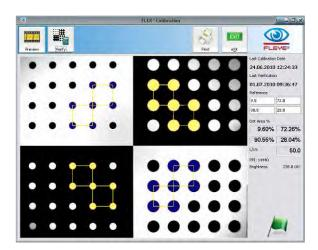
A horizontal and vertical red line guide the correct positioning of the calibration target. It is important that the image captured matches the expected image in order to ensure a valid calibration of the system.
