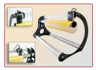
Dual transmission illuminators produce sharp, high-contrast images for accurate halftone dot analysis
