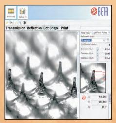
3D Imaging is the Only Way to Calibrate and Control HD Screening Techniques Photopolymer and elastomer plates are easily imaged, analyzed, and compared to the shop standard. The Pass/Fail indicator simplifies the production worker's job while detailed measurement data is available to the QC manager and
