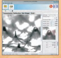
Using reflection illumination, plates are analyzed before or after mounting, flat on the bench, or mounted on the press. Plate wear and damage can now be evaluated before committing to running potentially bad plates.
