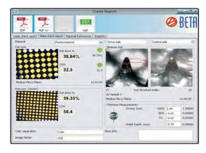
to communicate plate targets and tolerances, plate ID, and instrument settings. Reports and data are maintained in hot folders as well as output in user-selected formats.
