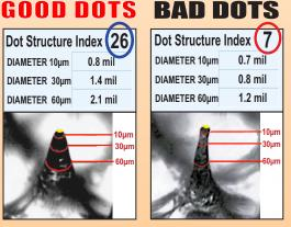
Dot Structure Index gives a simple one-number analysis of the dot shape, diameters at three points along the shoulder accurately describe the stability of the dot, and a reference and sample image comparator give a visual guide to the shape of the dot. Higher Dot Structure Index numbers show a better dot.
