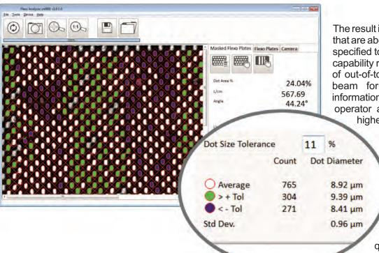
The result is a color coded display of cells that are above, below, or within the user-specified tolerance. This unique display capability reveals a vertical arrangement of out-of-tolerance cells, indicative of a beam formation error. Diagnostic information is instantly available to the operator and the technician, assuring highest quality and consistency.
