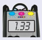
Measuring a specific process color will illuminate the corresponding flashing LED. Measuring Black or Gray Balance will simultaneously flash all 3 LED's.
