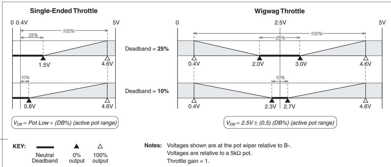
**Fig. 9** Effect of adjusting the throttle deadband parameter.
