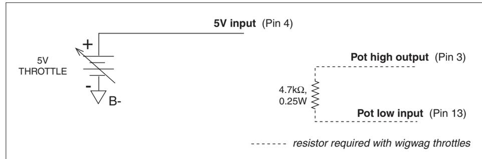
Voltage throttles with less than 5 V total voltage change over the full stroke can be accommodated by programming the controller for reduced-range throttle inputs, via the throttle gain parameter (see page 25).
