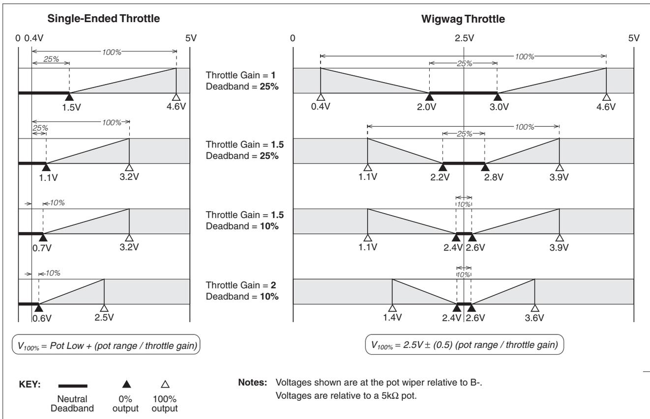
**Fig. 10** Effect of adjusting the throttle gain parameter.
