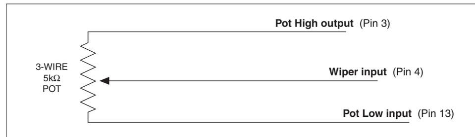
For wigwag and inverted wigwag applications, the pot can be correctly centered within the controller's neutral band by using the throttle autocalibration feature (see page 23). Pots with less than 5 k $\Omega$  total resistance change over the throttle's full stroke can be accommodated by programming the controller for reduced-range throttle inputs, via the throttle gain parameter (see page 25).
