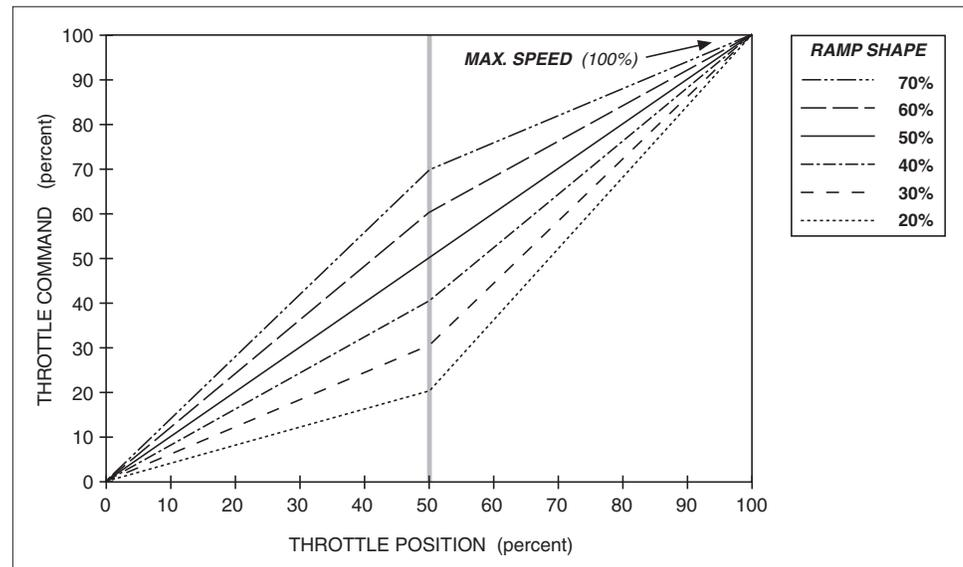
Changing the maximum speed setting changes the throttle command range, and hence the ramp shape. Ramp shapes with the maximum speed setting dropped from 100% to 60% are shown in Figure 12.
