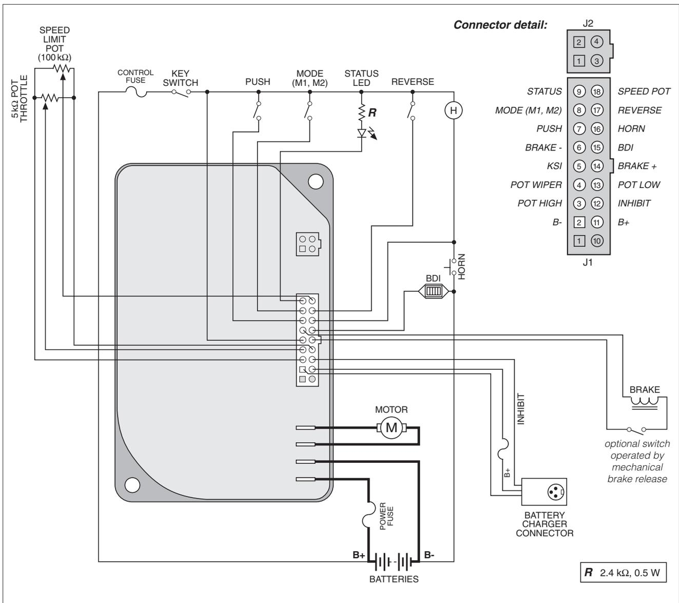
Fig. 3a Standard wiring configuration, Curtis 1210 controller.
