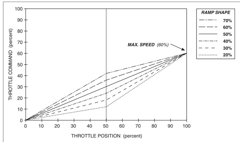
In all cases, the ramp shape number is the throttle command at half throttle. In Figure 12, for example, the 50% ramp shape results in a 30% throttle command at half throttle (i.e., a command that is halfway between 0% and 60%). The 20% ramp shape results in a 12% command at half throttle (20% of the range from 0% to 60%).
