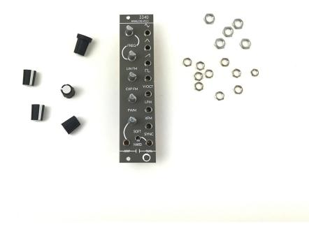
Affix the front panel to the jacks and pots using the included hex nuts. Once you've tightened them you can attach the knobs to the potentiometers by matching the cutout on the bottom of the knob with the position of the pot shaft, and pressing down.
