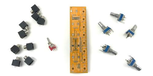
Populate the PCB with the 5 10k Potentiometers. They should be seated onto the top side of the PCB (easily verified by the boxes indicating the "M-10K-B" pots).
