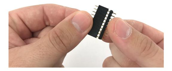
With the board face down, insert the female headers into the 6HP PCB.
