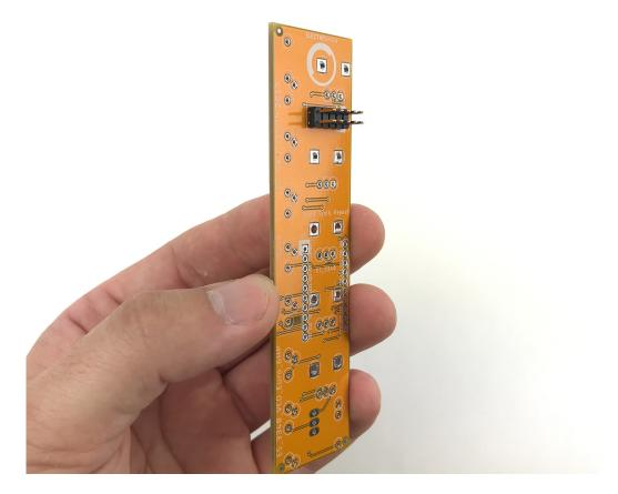
The side of the PCB with the red stripe notated is the bottom side of the PCB.
