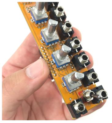
Install the front panel so that all of the jacks and pots fit into their holes.
