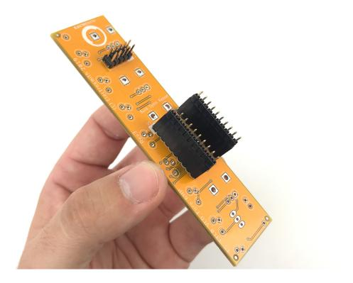
Place the Electrosmith 3340 submodule with pin 1 (indicated by a square pad) aligned with the marker on the 4hp PCB. The trim pot, and logo should be pointing up.
