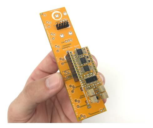
Flip the module over, leaning the now connected submodule against a surface that will keep all of the headers flush with the 4hp PCB.
