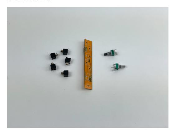
Populate the PCB with the 2 10k Potentiometers. They should be seated onto the top side of the PCB (easily verified by the boxes indicating the "M-10K-B pots).
