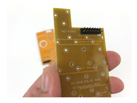
All of the connections that need to be soldered are highlighted with white circles to visually assist in the build process
