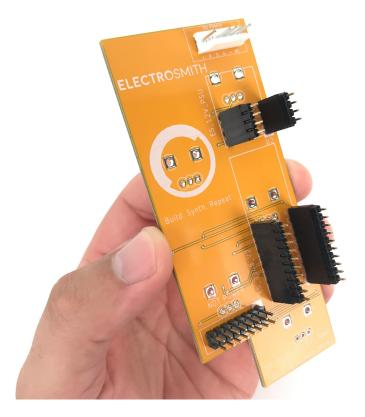
With the board face down, insert the female headers into the 1MU PCB.
