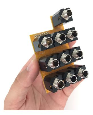
Install the front panel so that all of the jacks and pots fit into their holes.
