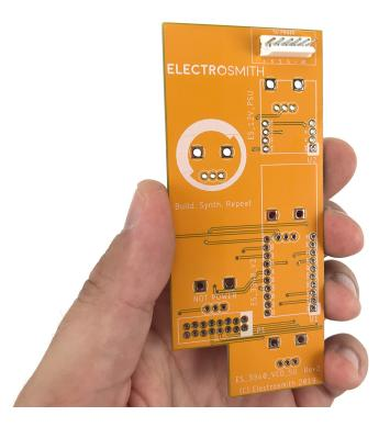
The side of the PCB with the text "5U POWER" is the bottom side of the PCB.
