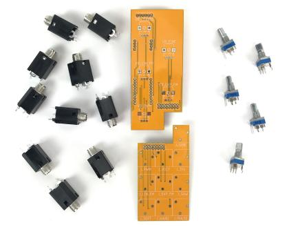
Populate the PCB with the 5 10k Potentiometers. They should be seated onto the top side of the PCB (easily verified by the boxes indicating the "M-10K-B pots).
