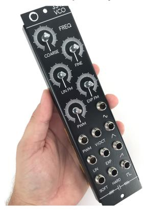
Flip the module over, and place the front panel on two objects of equal height to ensure that gravity is holding the PCB against the jacks.
