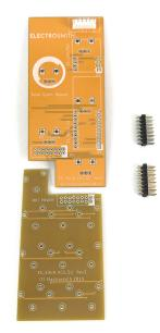
Populate both PCBs with the 2x8 male headers. The short pins should be pointing through to the top-side of the PCB, while the plastic and longer side of the pins should be visible on the back of the PCB.
