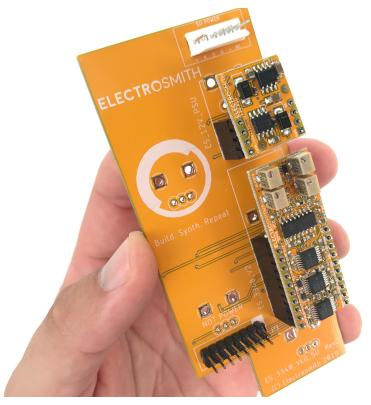
Flip the module over, leaning the now connected submodule against a surface that will keep all of the headers flush with the 1MU PCB.
