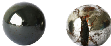
Ceramic ball vs steel ball after a hammer test
