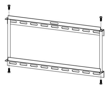
The long arms will attach to the back of your flat screen TV. All TV's come with the same mounting holes, this bracket is designed to be universal so that it works with all TV's and gives you flexibility to position the TV relative to the Lift however you prefer.
