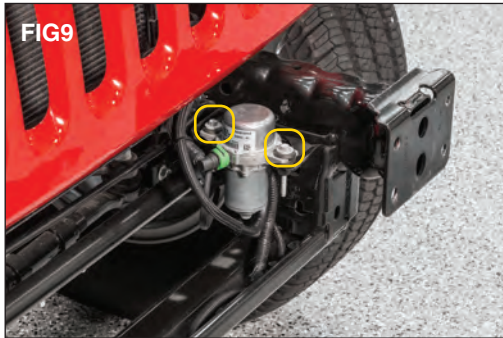
On 2012 and newer models locate and remove the mounting hardware for the brake vacuum canister using 10mm socket or wrench. (FIG 9)
