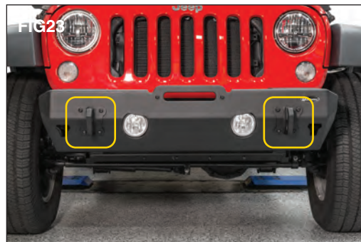
Loosely install the tow hooks through the bumper and into the winch plate with the supplied M10 allen head bolts and washers using a 6mm hex key. (FIG 23)
