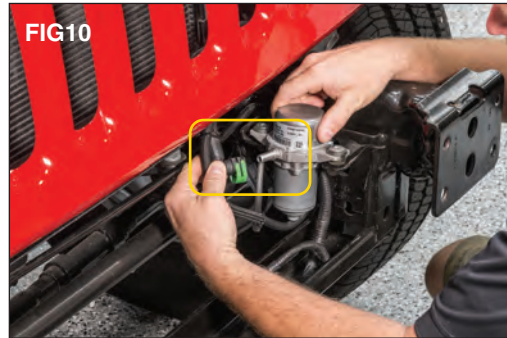
Slide down the green tab and slide off the large hose. (FIG 10)
