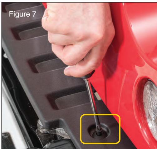
Remove the plastic screw rivets with a phillips screwdriver. (FIG7)
