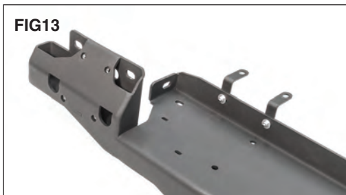
Install the canister brackets to the winch mount as shown with M6 washers and lock nuts using a 10mm socket. (FIG 13) This is shown upside down for illustration purposes.
