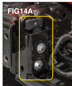
Loosely install the left and right nut plates to the inside of frame rails with the M10 x 20 Bolts and fender washers using a 17mm socket. (FIGs 14 A&B)
