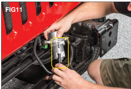
Pull of the small breather hose by pulling downward. (FIG 11)
