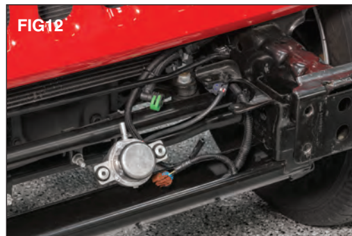
Carefully set canister out of the way. (FIG 12)
