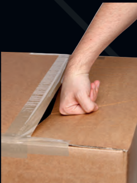
> pressure-sensitive tape separates from the carton under pressure.
