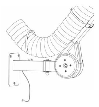
If the HPD has been installed using a boom extension use the hose straps provided to secure the hose ensuring the boom extension is free to pivot.
