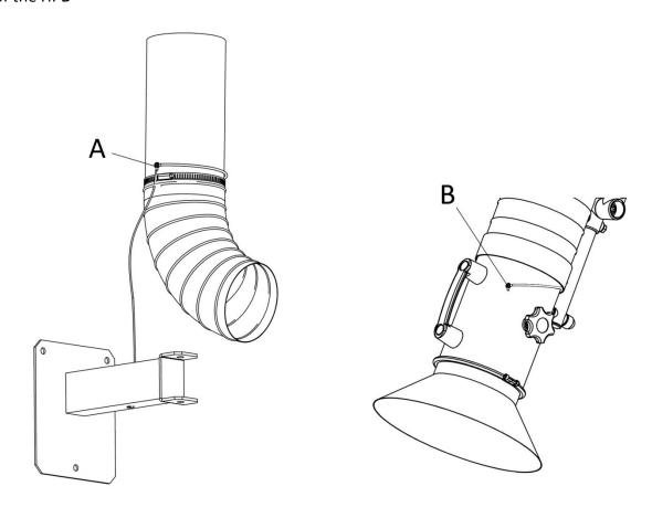
3) The continuity tester should indicate that there is a circuit present between the duct connection (A) and the hood (B). If no circuit is indicated as present, then there is a break in the spiral hose which must be replaced immediately. Contact flextraction with the details of the product serial number to ensure that the correct replacement hose is ordered.
