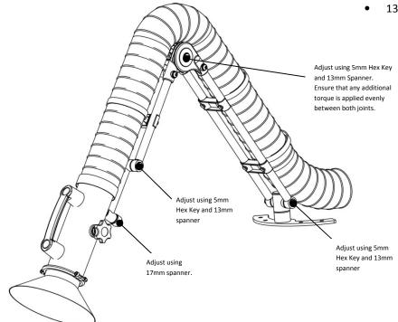
1d) Installation of the boom extension system (4m/5m - if supplied);
