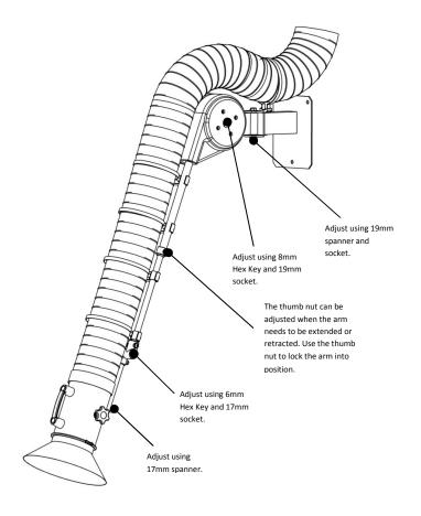
To adjust the telescopic HPD the following tools will be required;
