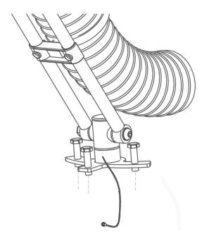
Install the bench mounting bracket using 3 x M8 bolts, It is recommended that the mini HPD is installed within 0.4m of the duct connection.
