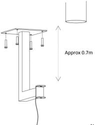
It is recommended that the ceiling bracket is installed within 0.7m of the duct connection.
