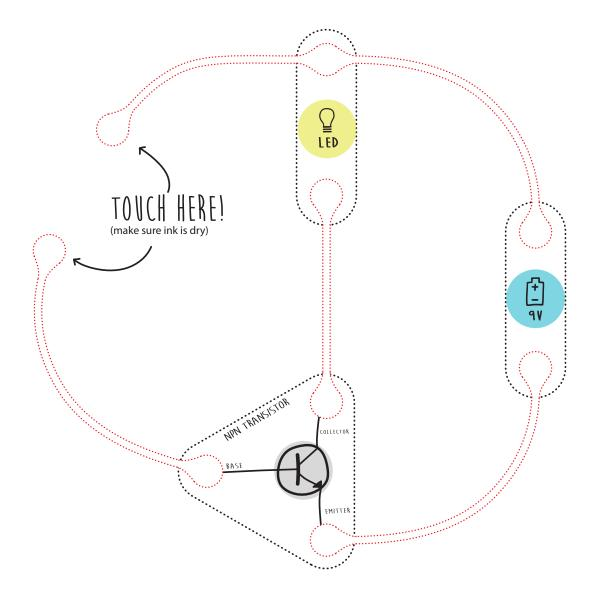
**Tip:** Remove the Transistor and put a Switch where the collector and emitter feet go. Do you see how both modules are a type of switch?
