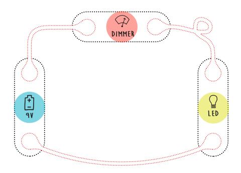
**Tip:** The Circuit Scribe ink conducts easily, with a resistance of only about 1 ohm per centimeter.
