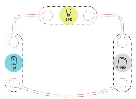
Resistance is measured in **ohms**. Higher resistance = lower current and a dimmer LED.
