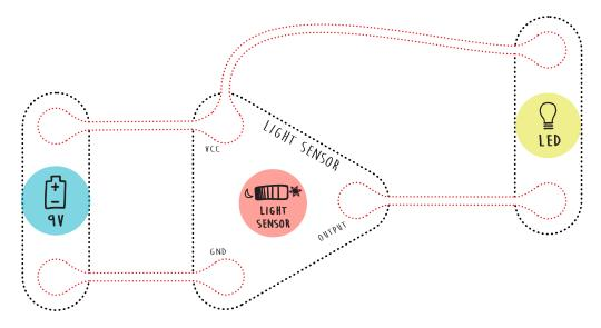
**Tip:** The Light Sensor is a "photo transistor." Instead of responding to a small electrical current, it amplifies or switches in response to light. Learn more about the Light Sensor at **sketch.circuitscribe.com**.
