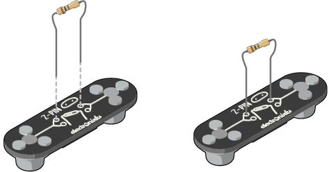
After drawing the circuit, swap in different resistors and watch the change in LED brightness. See if you can line up the resistors based on their conductivity!
