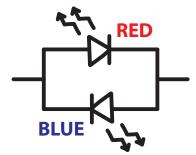
Our LED module has 2 LEDs wired up in opposite directions. Flip the module around to switch its color between red and blue.
