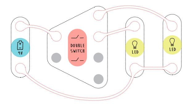
The circuit above only uses the top of the Double Switch. This switch is actually two separate toggle switches controlled by one lever. It can control not just one, but two circuits!
