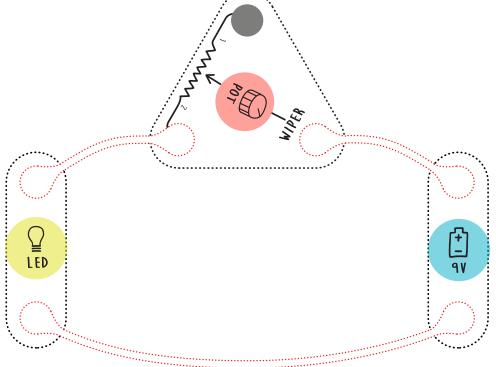
**Tip:** Always use the wiper foot in your circuit – peek under the knob opposite the squiggly line to see the "wiper" label.
