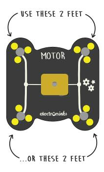
**Or try the motor!** Replace the LED above with the Motor Module. Flip the switch to change the direction that the motor spins.
