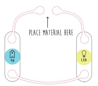
Leave a gap in the circuit above. Press materials from around your home or classroom over the gap to "close" the circuit.
