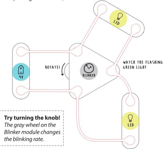
The LEDs in the circuit are connected in two different ways. Do you see the difference after you complete the circuit?
