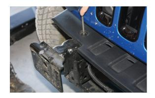
**6.** If equipped with factory fog lights, those may be removed from the stock front bumper and install the new front bumper with the supplied mounting hardware.
