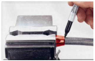
**Step 3:** It is important to mark the outside of the hose at the end of the socket. This will show you if the hose has "pushed out" of the socket during assembly, and if so, will leak when used.
