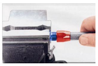
**Step 5:** Hold the hose and not the socket, start the hose on the nipple of the hose end, with a gentle motion. Continue pushing on the hose until the threads can be engaged. Some sizes may require the use of some force to engage the threads at this point.
