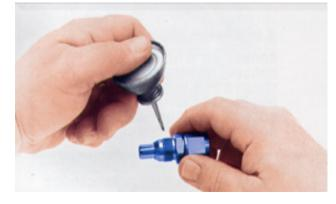
**Step 4:** It is very important to lubricate the inside of the hose/socket assembly, and the outside of the cutter threads with any assembly lube, anti-seize compound, or 30 wt. Motor Oil. W/D-40 is not recommended!
