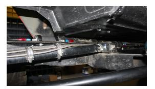
Mount fuel pump on frame, the lowest point the better, which will help fuel pump stay primed.
