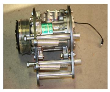
Install assembly onto the engine and install serpetine belt tensioner with the M10 x 1.5 x 170 mm long bolt, flat washer, and lock nut. Once positioned, torque all hardware.
