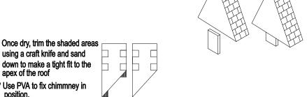
Glue in small 3mm blocks to inside of gables leaving 5-10mm protruding
