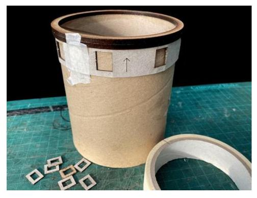
Align one window centrally above the door then tape in place. Next, glue each window to the card tube and remove the spacing strip.
