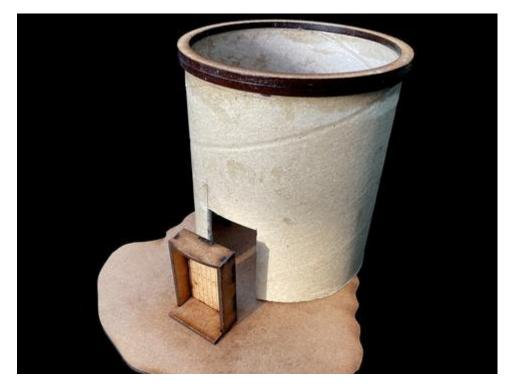
Glue on the thinner 3mm ring around the top lip of the tube then glue on the thicker 3mm ring to cover this and the tube top edge. DO NOT glue the card to the base yet.
