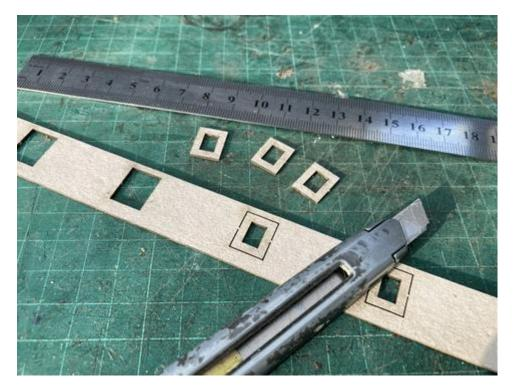
Cut the window frames from the card strips and set aside. Using tape, join the two strips to make one long length.
